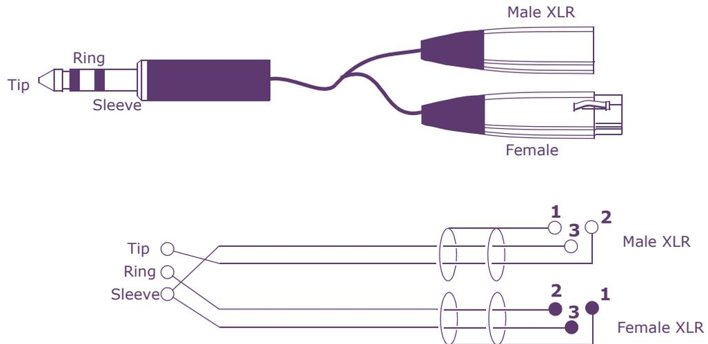
Figure 3: Insert send/return 1/4" TRS connector/XLRs - wiring details
