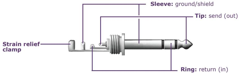
**Note:** Connect insert send with input and insert return with output of effects device.
