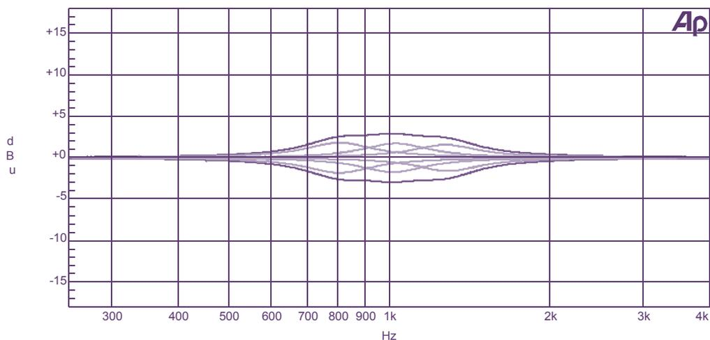
Figure 4: Constant-Q equaliser 'wide' mode  $\pm 2$ dB boost and cut
