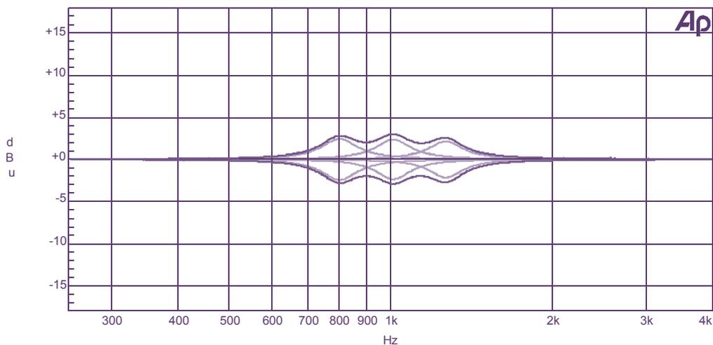
Figure 5: Constant-Q equaliser 'narrow' mode  $\pm 2$ dB boost and cut
