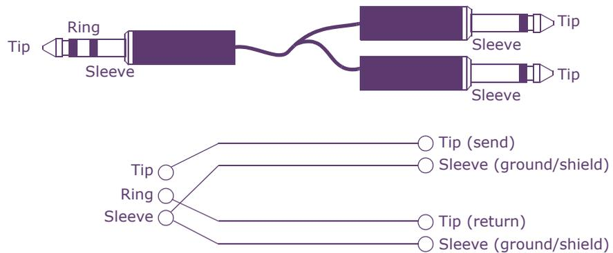
Figure 2: Insert send/return 1/4" TRS connectors - wiring details
