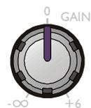
The gain control provides continuous adjustment of the channel gain from minus infinity (off) to +6dB with a centre detent at 0dB (unity gain). When using EQ with large amounts of cut or boost, it may be necessary to use the gain to make up or attenuate the signal.
