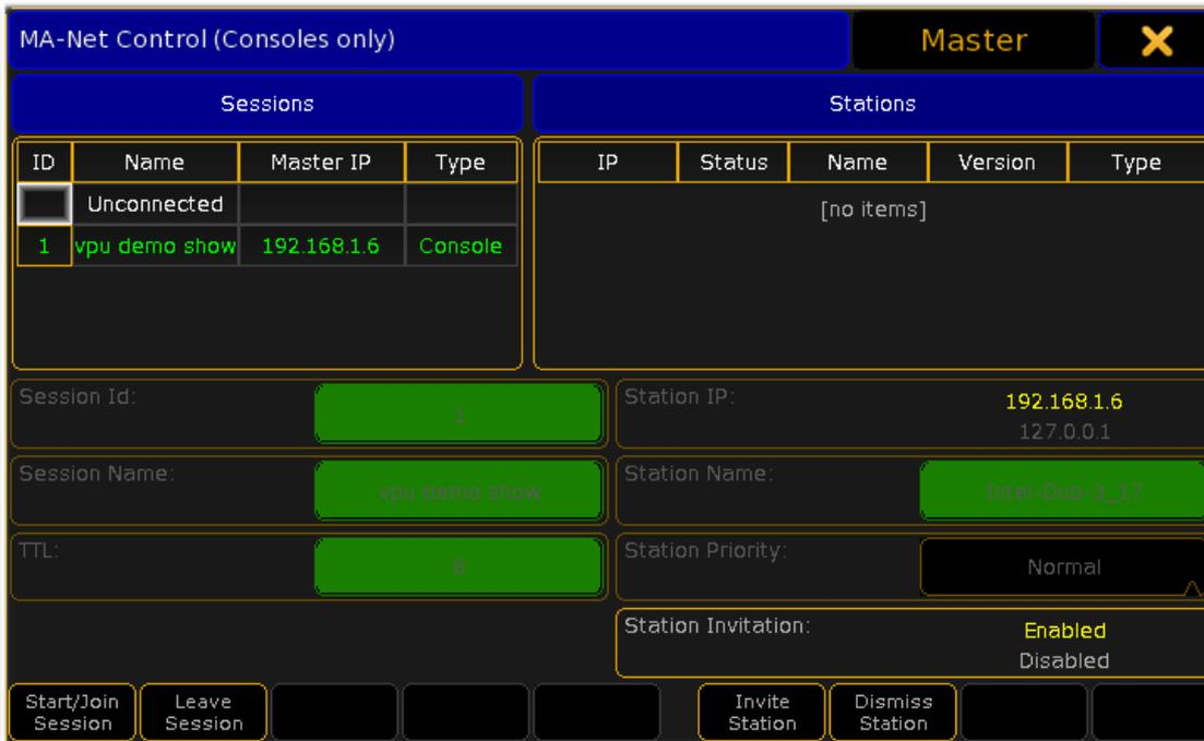
Press 'Setup' select the tab 'Network Standalone' and press 'MA Network Configuration'
