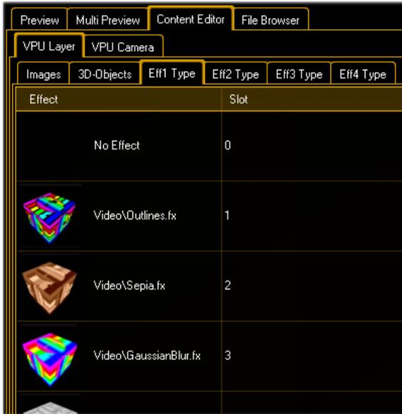
The effect engine is based on the Direct3D standard. Effects are defined within .fx files. An effect file is a text file with an .fx extension. It defines how something is to be rendered. It includes state information along with vertex and shader declarations. The shader code is written in HLSL (High Level Shading Language). The following example shows the assignment of a sepia effect the test image:
