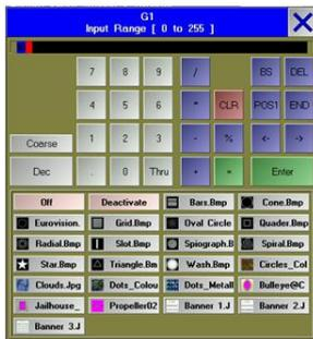
If you want to change the image or video for the layer, scroll through the image selection with the encoder wheel or select the image or video from dialog after clicking on the image entry.
