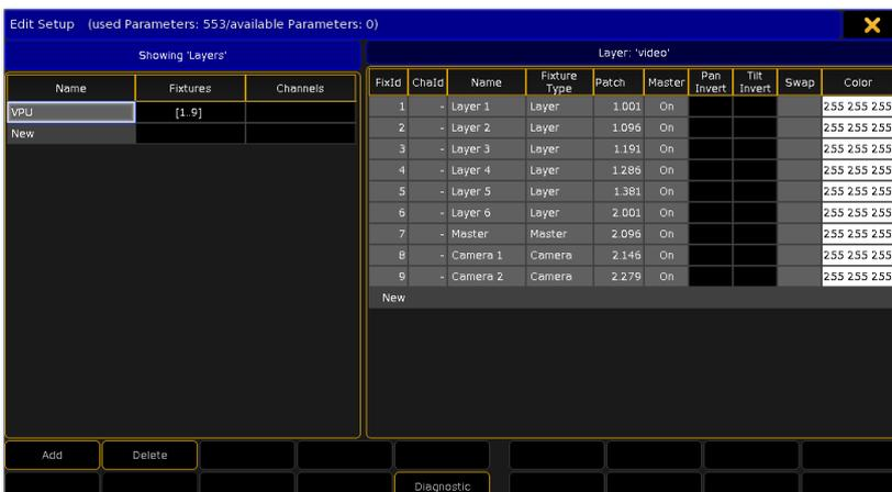
A layer in MA VPU is analog to a Fixture in the grandMA desk.
