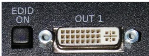
The switch near the DVI OUT connector lights **blue** if EDID is simulated.
